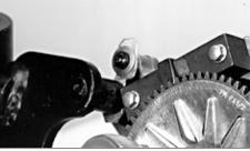
Make careful note of where this tool comes level with the starter ring gear plate of the starter motor in order to make sure, when refitting, that the pressure plate fits correcte into the grooves of the crankshaft.
